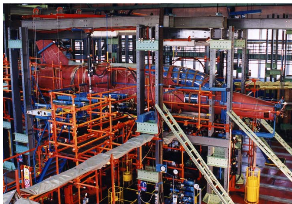
Full-scale fatigue tests of commuter and light combat aircraft completed by VZLU
