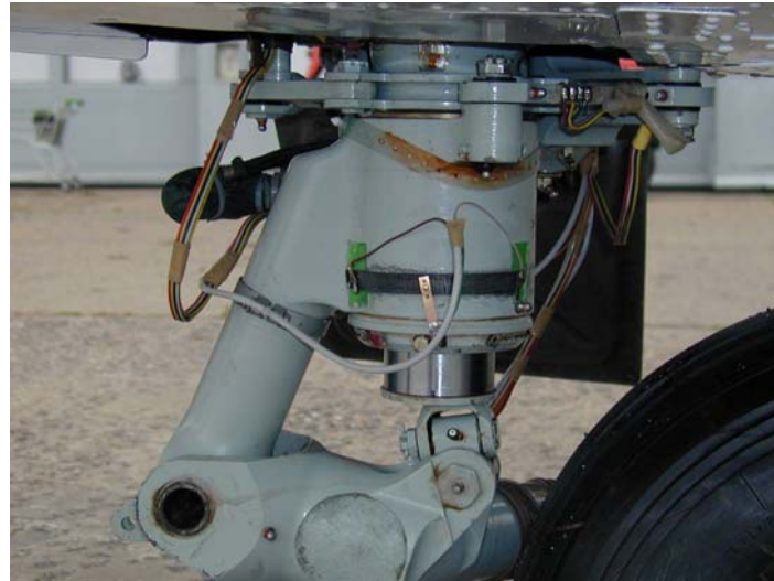
Nose landing gear of L-410 Commuter
