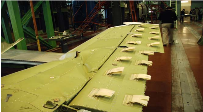
Example of wing buckling
